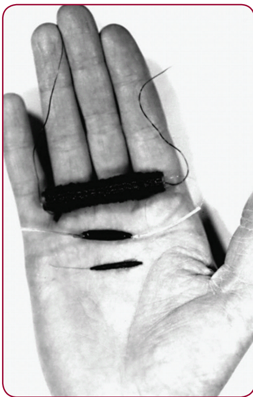
FIGURE 1-8. An example of induction coils used by Charles Eyriès and André Djourno. Image provided courtesy of Claude-Henri Chouard, M.D.
